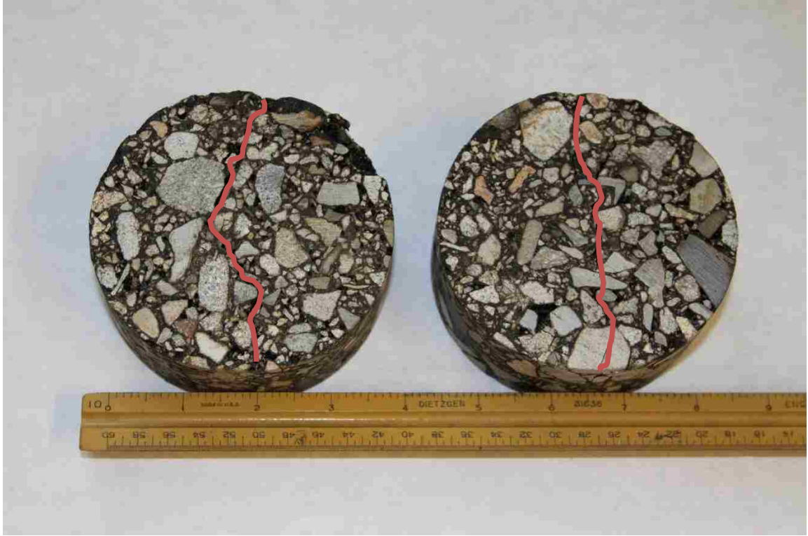
Figure 4.3. Asphalt Cylinder Specimens after Completion of IDT Test
